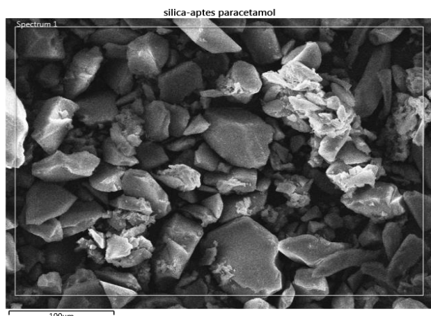
Figure 3b: Shows SEM Images of activated silica after modification.
